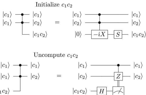
**Figure 4:** Gidney’s [3] 4-T “Temporary logical-AND” construction, consisting of two circuits extended from Jones’ Toffoli [7]. The first circuit computes the product  $c_1c_2$  onto an ancilla, and the second circuit uncomputes it. The product can be copied from the wire between the two circuits and used for other computations.
