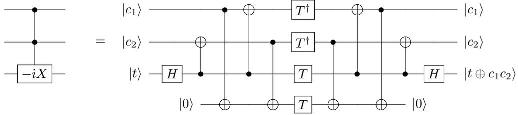
**Figure 2:** Selinger’s [10] doubly-controlled  $-iX$  gate, implemented with 4 T gates. This gate achieves the effect of a Toffoli and contributes a global phase of  $i$  to the target qubit if both controls are  $|1\rangle$ .
