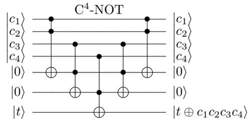
Generalizing this pattern, a circuit for  $n$  controls requires  $2n - 3$  Toffolis. At 4 T gates per Toffoli, we obtain an upper bound on the  $C^n$ -NOT T-count of  $8n - 12$ . This count is already favorable, as it only grows linearly as controls are added.
