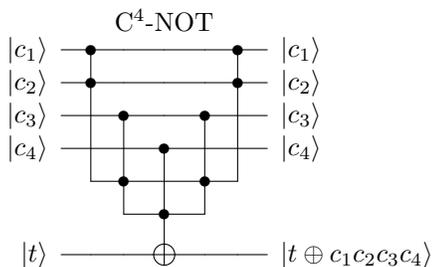
Each pair of Toffolis on the same wires from the previous circuit is replaced by a temporary logical-AND. Since each logical-AND can be computed and uncomputed for the T-count of only one Toffoli, we effectively almost half the T-count of the entire circuit (the “almost” comes from fact that the central Toffoli on the target qubit remains from the previous construction). Precisely, the new count is 4 T times  $n - 1$  Toffolis for  $4n - 4$  T.
