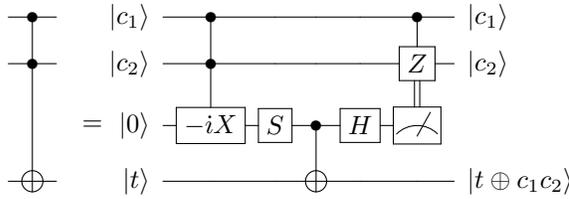
**Figure 3:** Jones’ [7] Toffoli circuit, implemented with 4 T gates. It works by 1.) targeting an ancilla with a doubly-controlled  $-iX$  gate, then correcting the  $i$  phase with an S gate; 2.) XORing the  $c_1c_2$  product onto the target qubit with a CNOT; then 3.) uncomputing the ancilla with a Hadamard and measurement-controlled CZ gate.
