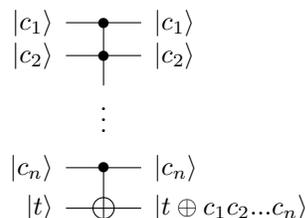
**Figure 1:** A  $C^n$ -NOT gate. The product  $c_1 c_2 \dots c_n$  is added to the target qubit state, modulo 2. Gates of this type are used to implement classical reversible functions in the quantum context.
